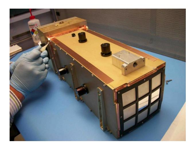
Integrated instrument prototype with the optics assembly at the front and the electronics box in the back. Credit: NASA
