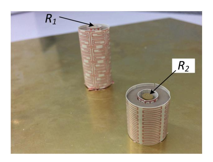
The fabricated metasurface material for antennas, created by Werner and Jiang. Credit: Penn State
