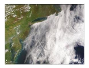
Satellite image of ship tracks, clouds created by the exhaust of ship smokestacks. Image: NASA
