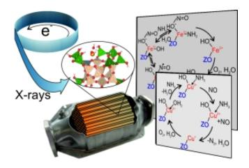
With the help of X-rays, reactions in catalytic converters can be observed under close-to-reality conditions. Credit: KIT-ITCP
