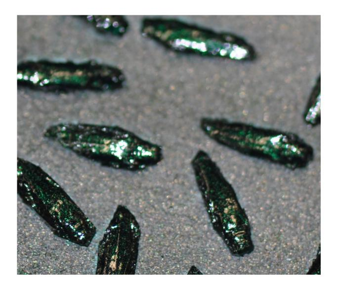
Ash borer decoys produced in a single die by the heat-cured plastic method developed by engineers at Penn State and Western Michigan University. The decoys, which mimic female ash borers, have proven to be effective at attracting
