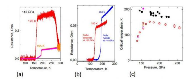
Pressure and temperature effects on Tc in sulfur hydride and sulfur deuteride. Credit: arXiv:1506.08190 [cond-mat.supr-con]
