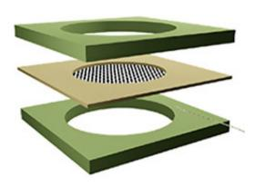
An atom-thick layer of carbon atoms, called graphene (black mesh), provides the vibrating diaphragm for both an ultrasonic microphone and loudspeaker. Credit: UC Berkeley image.
