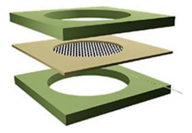
An atom-thick layer of carbon atoms, called graphene (black mesh), provides the vibrating diaphragm for both an ultrasonic microphone and loudspeaker. Credit: UC Berkeley image.
