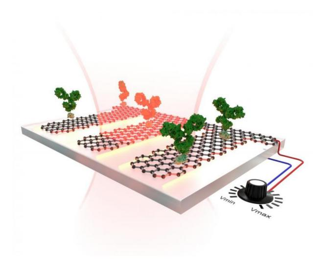
Making graphene's electrons oscillate in different ways makes it possible to "read" all the vibrations of the molecule on its surface. Credit: *Science* / EPFL / Miguel Spuch / Daniel Rodrigo
