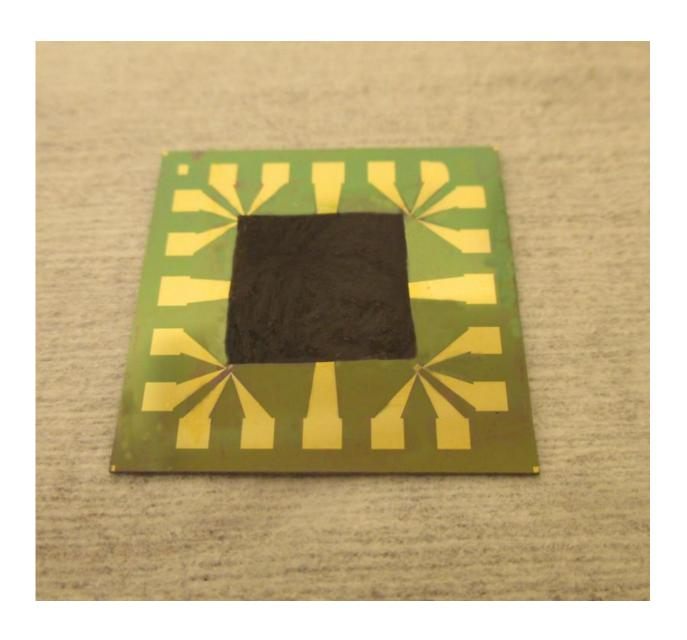
Graphene-based film on an electronic component with high heat intensity. Credit: Johan Liu / Chalmers University of Technology
