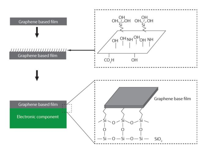
Silane coupling between the graphene and the silicon (an electronic component). After heating and hydrolysis of (3-Aminopropyl) triethoxysilane (APTES)
