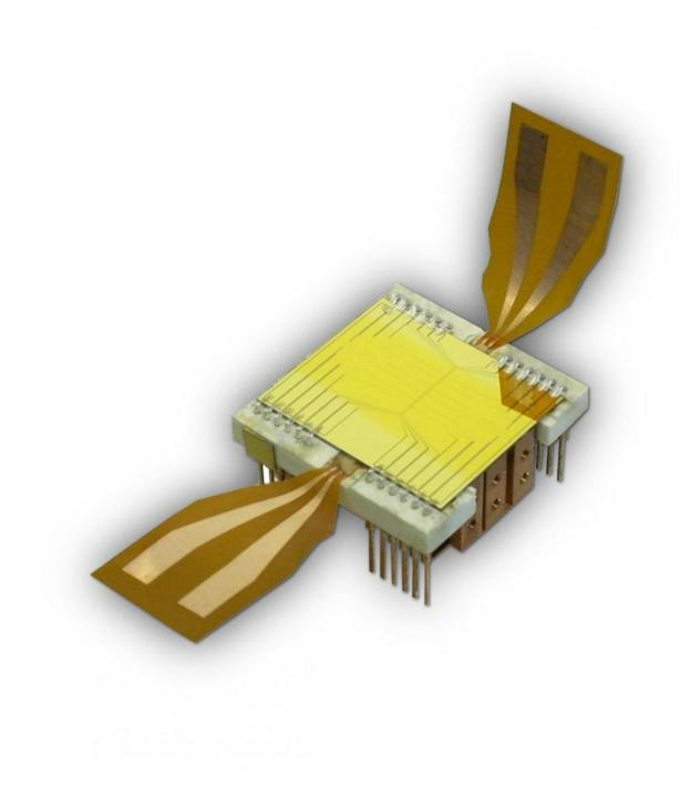
The atom chip used to control the atoms. Credit: TU Wien
