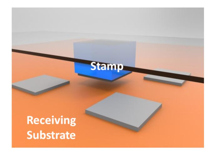
Laser micro-transfer printing constructs micro- and nanocircuits from conventionally fabricated microstructures without contact between these fragile assemblies. In this illustration of the beginning of the process, the stamp (blue) with nano "ink" (grey) goes to position over the receiving surface (orange). Credit: Jorge E. Correa and Placid M. Ferreira, mechanical science and engineering, University of Illinois at Urbana-Champaign
