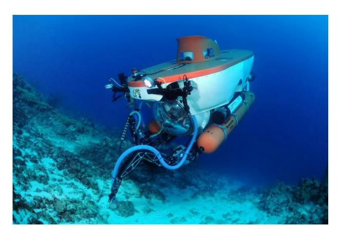
The Curasub is a five-person submersible capable of descending to 300 m (1,000 ft.) and equipped with hydraulic robotic arms useful in collecting biological samples. Credit: Barry Brown, Substation Curacao
