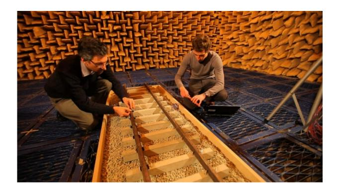
Scale track model tests for noise radiation and absorption. Credit: University of Southampton
