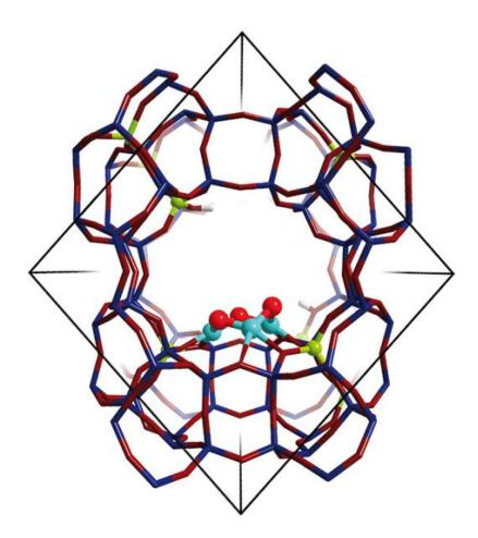
A new bio-inspired zeolite catalyst might pave the way to small scale "gas-toliquid" technologies converting natural gas to fuels and starting materials for the chemical industry. The copper exchanged zeolite with mordenite structure mimics the reactivity of the enzyme methane monooxygenase (MMO). Credit: Guanna Li and Evgeny Pidko / TUe
