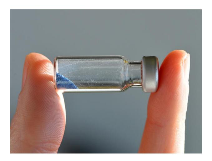
A new bio-inspired zeolite catalyst might pave the way to small scale "gas-toliquid" technologies converting natural gas to fuels and starting materials for the chemical industry. The copper atoms provide the zeolite with a bluish color Credit: Andreas Battenberg / TU München
