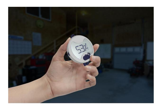
Mexican startup Brain Fusion, which specializes in the Internet of Things (IoT), has designed a device for smartphones and tablets that monitors in real time the amount of gas from a stationary tank,
