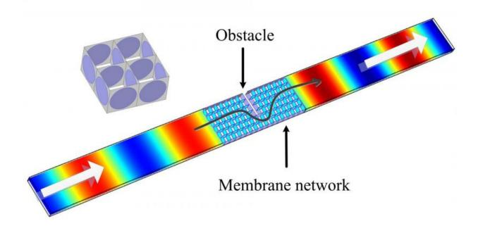
Schematic representation of sound passing through the density-near-zero membrane. Credit: Liu/Nanjing University
