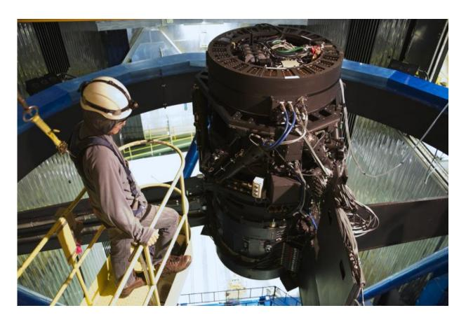
Figure 2: Hyper Suprime-Cam at Subaru telescope's prime focus. Credit: NAOJ/HSC Project
