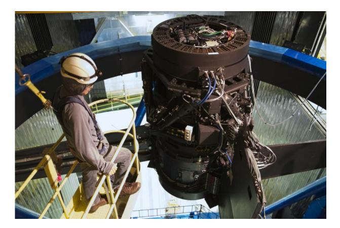
Figure 2: Hyper Suprime-Cam at Subaru telescope's prime focus. Credit: NAOJ/HSC Project
