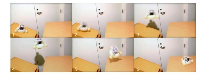
In a series of tests, the robot jumped two and a half feet (0.75 m) in height and half a foot (0.15m) laterally. In experiments, the robot jumped more than 100 times and survived an additional 35 falls from a height of almost four feet. Credit: Jacobs School of Engineering/UC San Diego/Harvard University
