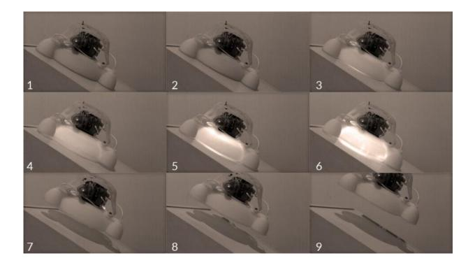
The robot is capable of more than 30 untethered jumps and is powered by a mix of butane and oxygen. Credit: UC San Diego/Harvard University
