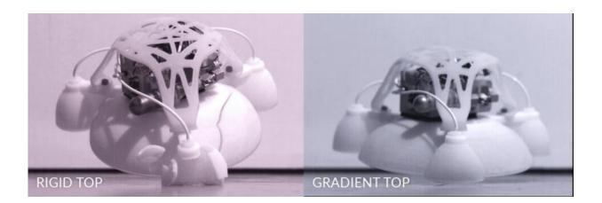
Left: the rigid top fractures on landing, while the top made of nine layers going from rigid to flexible remains intact. Credit: Jacobs School of Engineering/UC San Diego/Harvard University
