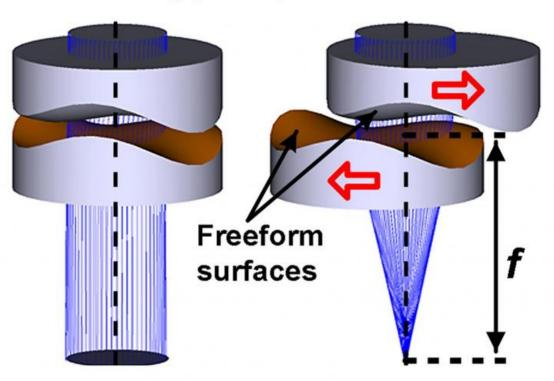
The miniature solid tunable lens technology may enable compact optical zoom endoscope with autofocus capability that could switch conveniently from a wide field-of-view to a clear high-resolution close-up view without moving the endoscope probe. Credit: Zhou Guangya, National University Singapore
