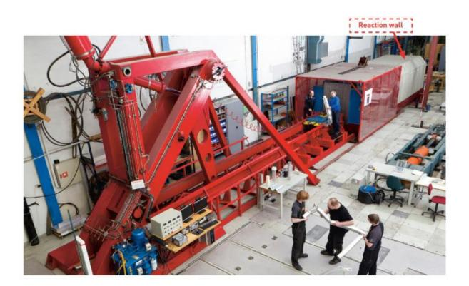
The pendulum accelerator, otherwise known as the "kicking maching" is the largest machine of its type in the world. The kicking machine is designed to deliver high impact, high velocity blows to whatever material scientists want to test. The machine is also outfitted with a high-speed camera so researchers can conduct frame by frame analysis of what has happened during the collision. Credit: Ole Morten Melgård
