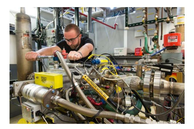
Argonne researcher Jim Sevik tightens the fuel rail on a natural gas directinjection system at the lab. The engine is an automotive size single-cylinder research engine that operates with gasoline as well as natural gas.
