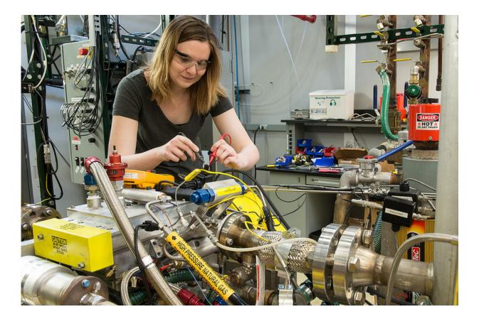
Visiting IIT Professor Carrie Hall troubleshoots the engine wiring harness. The Argonne system can replicate speed and load conditions found during typical vehicle operation for both naturally aspirated as well as turbocharged engines.
