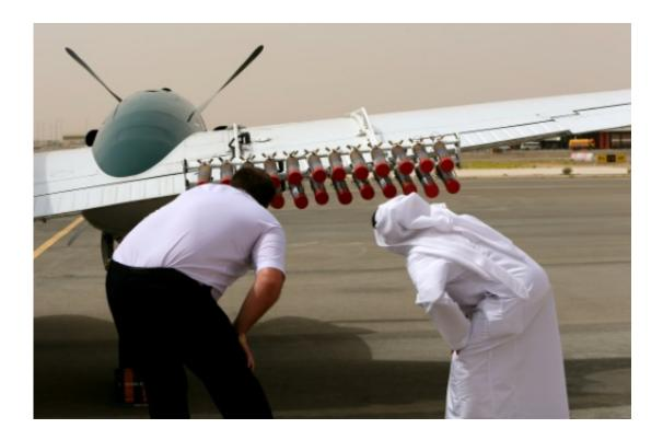
A pilot and a UAE official from the national center for meteorology and seismology check salt flares at al-Ain airport that are fired into a promising cloud to increase condensation and hopefully trigger rainfall
