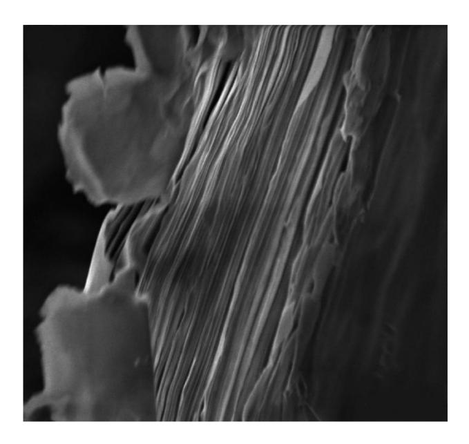
This is a scanning electron microscopy image of stacked clay sheets. When twodimensional sheets of the clay, called vermiculite, are exfoliated in water, they carry negative charges, attracting positively charged protons. After the sheets
