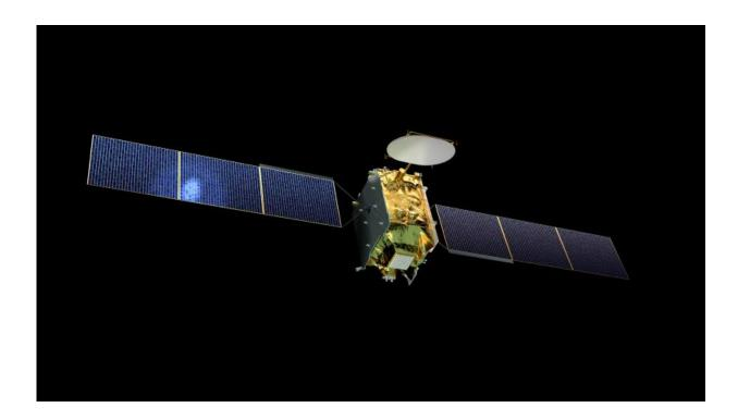
Quantum represents a shift from custom-designed, one-off payloads to a more generic approach, resulting in reduced cost and time through a modular and scalable answer to the payload specification, design, technology and manufacturing. It will also be capable of unprecedented in-orbit reconfigurability in coverage, frequency and power, allowing complete mission rehaul, including orbital position. Credit: Airbus
