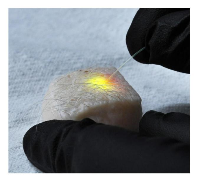
Inserting an optical fibre into a piece of pig's skin to excite and extract the laser light generated by subcutaneous fat cells. Credit: Matjaž Humar and Seok Hyun Yun, CC BY-ND
