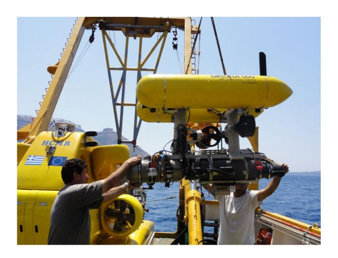
The crew from the R/V Aegaeo ready the University of Girona's autonomous underwater vehicle (AUV) Girona 500. Researchers used the AUV, equipped with the TETHYS mass spectrometer (shown strapped to hull), to identify subsea layers of water with unusual chemical properties. HCMR's Thetis sub is shown to the left and the island of Santorini is in the background. Credit: David Ribas,
