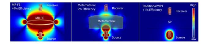
From left to right: performance of wireless power transfer using an MRFE, a metamaterial, and through air alone.
