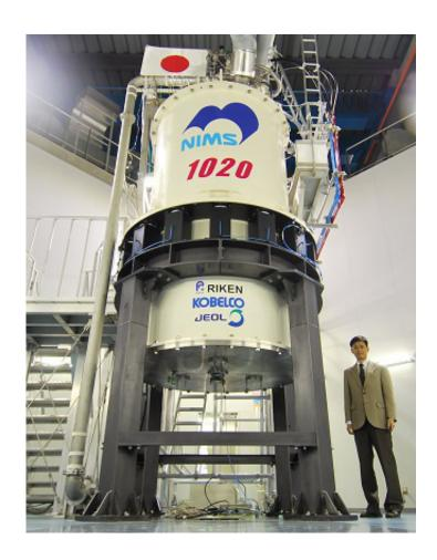
A part of the recently developed 1,020 MHz-NMR system equipped with superconducting magnets (about 5 m high and weighing about 15 tons). This part contains coils made of a high-temperature superconductor. Liquid helium is used for cooling.
