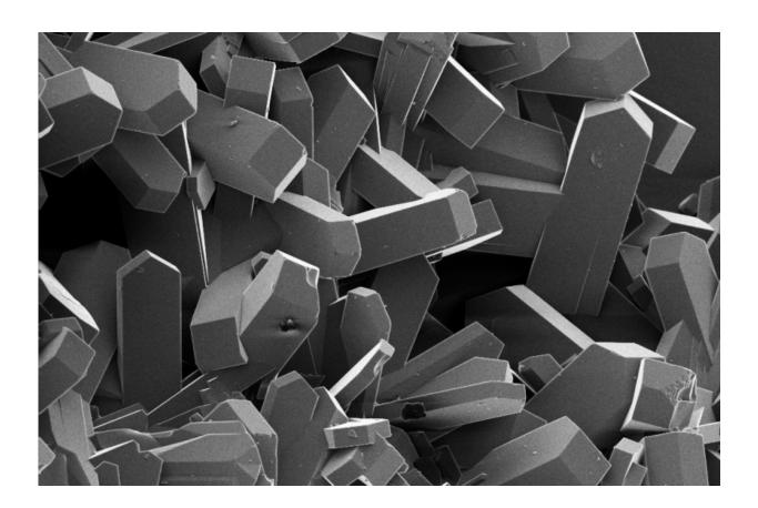
These coffin-shaped growths make up one variety of porous materials called zeolites. An international team of scientists discovered that when aluminum atoms in the material cluster in the overlapping intersections of these sub-units, zeolites lose their ability to convert oil to gasoline and other chemicals. Credit: PNNL
