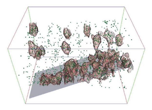
Green dots in this image represent aluminum atoms within a zeolite crystal. When aluminum atoms bunch up, zeolites lose their ability to convert oil to gasoline and other chemicals. An international team of scientists created the first 3-D atomic map of the material in order to find out how to extend the catalyst's life. Credit: PNNL
