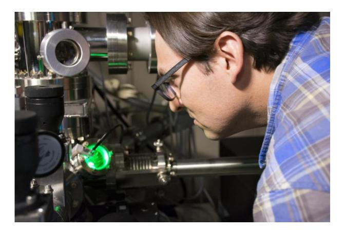
Pacific Northwest National Laboratory materials scientist Danny Perea looks into an atom probe, which he and an international team of scientists used to locate aluminum clusters responsible for the shutdown of catalytic activity in zeolites, a material used by industry to produce fuel and other chemicals. Credit: PNNL
