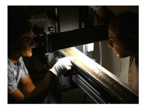
Setting up the core in multi sensor core logger (MSCL) at the paleoceanography lab at the Rosenstiel School, to make a high-resolution image and measure the physical properties such as density and magnetic susceptibility. Credit: Diana Udel, UM Rosenstiel School Communications Office
