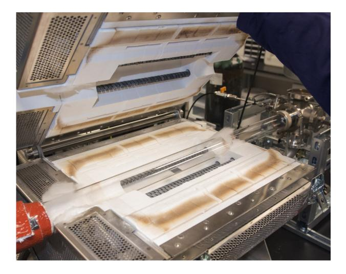
Inside the vapor deposition furnace, a quartz tube provides a controlled environment for the formation of 2D materials from vaporized organo-metallic compounds. Credit: Patrick Mansell, Penn State
