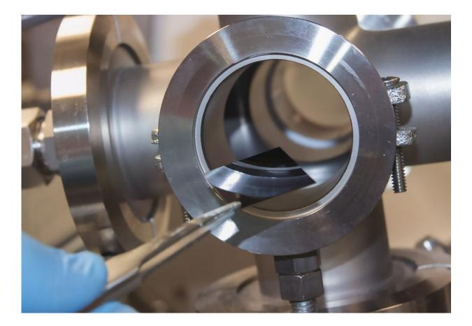
A silicon wafer, shown here being inserted into a tube leading to the vapor deposition furnace, will serve as a substrate on which new 2D materials can grow. Credit: Patrick Mansell, Penn State
