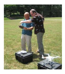
It takes two to use a quadcopter for research—one to fly the device (using the controller on the case) and a second to work a tablet, used for switching functions and monitoring the on-board camera. Gerard Chouin gives Sean Pada a little shade to get things started. Credit: Joseph McClain
