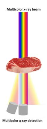
When x-rays go through an object, some of the radiations will be absorbed, some will be transmitted, and the last part will be scattered in different positions because of the interaction with atoms in the object. This reveals information about the structure of the object, for example connective tissues structure and muscle fibres. Credit: SINTEF
