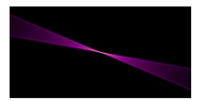
A reconstruction of the focused X-ray wave. The lens achieves the spot size of 8 nanometers at the smallest waist. Credit: Saša Bajt/DESY
