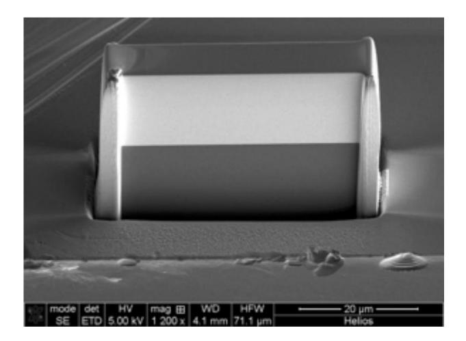
A scanning electron microscope image of the novel X-ray lens. The bright area is built from 5500 alternating layers of tungsten and silicon carbide. The dark area is the substrate. The width of the lens is 40 micrometers. Credit: Saša Bajt/DESY
