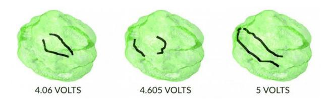
The 3D X-ray imaging technique used in the study shows how the defects move around inside the LNMO spinel as the battery is charged to higher voltages. Credit: Andrew Ulvestad/Department of Physics, Jacobs School of Engineering/UC San Diego
