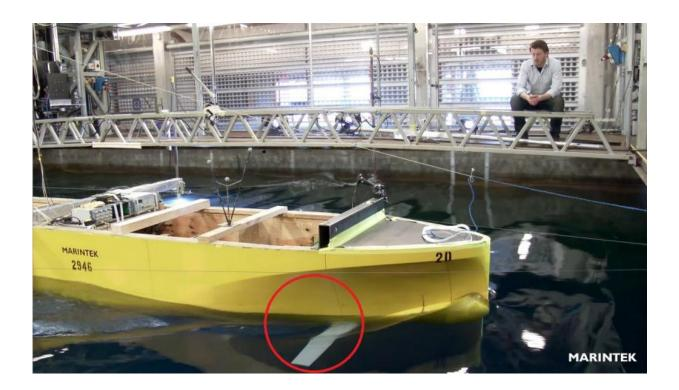
Eirik Bøckmann testing a ship with an artificial whale tail at the Marintek Towing Tank. Credit: Ingrid Snøfugl, Siw Hermanstad, Marintek/SINTEF
