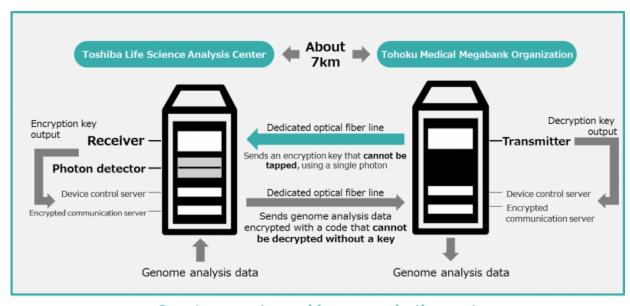
Quantum cryptographic communication system
