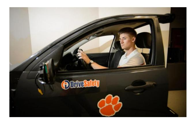
Researcher Drew Morris demonstrates how a Clemson vehicle simulator is used to measure driver fatigue. Credit: Ashley Jones
