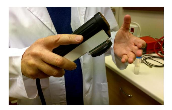
Prototype of the device which will allow bacterial meningitis to be diagnosed in babies in seconds with a high-resolution ultrasound of the fontanelle. The team is now working on making it smaller. Credit: Research Laboratory of Electronics
