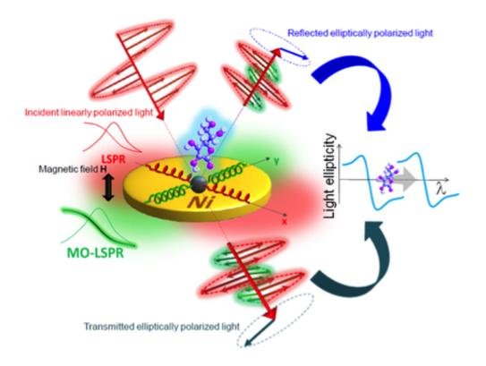
Light polarization manipulation enabled by phase compensation in the electric response of a magneto-plasmonic nanoantenna controlled through precise design of the LPRS resonance induced by the magneto-optical activity (MO-LSPR) of the ferromagnetic constituent material (Ni) and exploitation of the effect for ultrasensitive molecular sensing.
