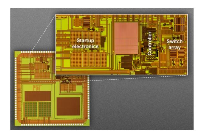
The MIT researchers' prototype for a chip measuring 3 millimeters by 3 millimeters. The magnified detail shows the chip's main control circuitry, including the startup electronics; the controller that determines whether to charge the battery, power a device, or both; and the array of switches that control current flow to an external inductor coil. This active area measures just 2.2 millimeters by 1.1 millimeters.
