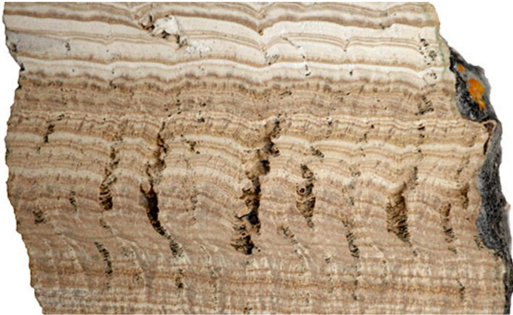
A cross-section of travertine, formed from limestone deposits in water flowing through the aqueduct.
