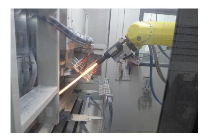
Thermal Spray Technologies uses a supersonic spray process to deposit a coating just a few thousandths of an inch thick at temperatures in the thousands of degrees. Here, the coating will alter the electrical properties of an innovative surgical device. Credit: David Tenenbaum
