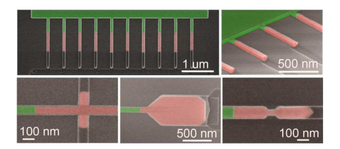
Scanning electron microscope images of single crystal structures fabricated using template-assisted selective epitaxy are shown. For better visibility, the silicon is colored in green, and the compound semiconductor in red. Credit: H. Schmid/IBM
