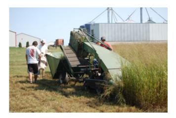
Harvesting switchgrass biomass samples with a flail harvester. Machine cuts and picks up biomass, blows it through a chute, weighs the biomass, and dumps in a wagon. Students pull random samples for dry matter determination. Credit: M.
