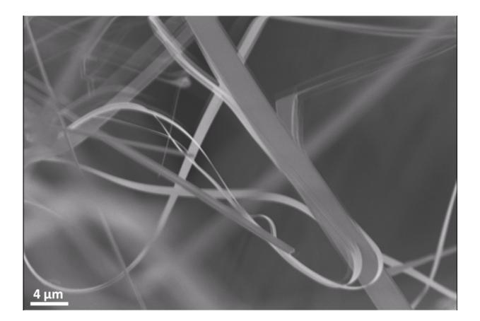
Pasta like SnO<sub>2</sub> structures vibrating under the electron beam of the electron microscope. Credit: Mishra/Wiley-VCH
