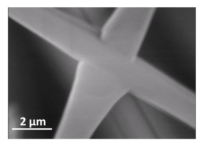
Interpenetration point of two crossing SnO<sub>2</sub> structures in defined crystallographic directions. Credit: Mishra/Wiley-VCH
