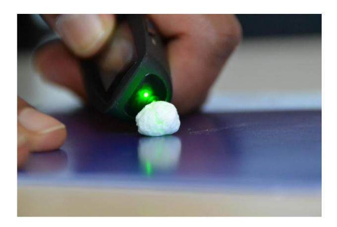
Just like wool made of fettucine: stretchable ceramic made from tin oxide shows the future of nanostructure growth. Credit: Claudia Eulitz, CAU
