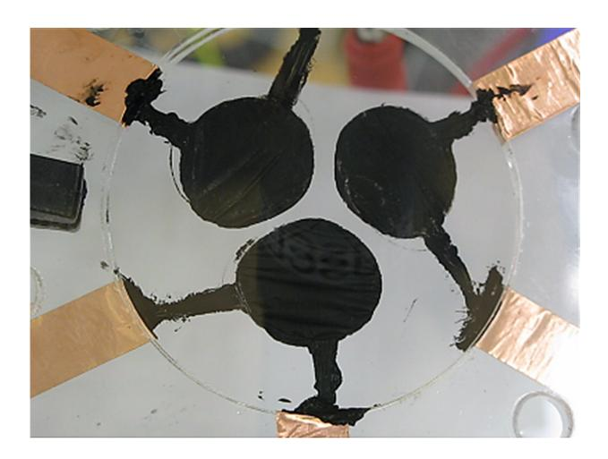
Three prototype artificial cephalopod chromatophores are shown in unactuated states. The chromatophores are made from dielectric elastomer using tape coated with black carbon grease electrodes. Credit: University of Bristol
