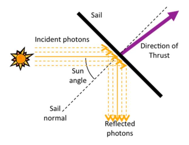
A solar sail produces thrust without propellant mass by simply reflecting incident photons from the sun. Credit: www.deorbitsail.com
