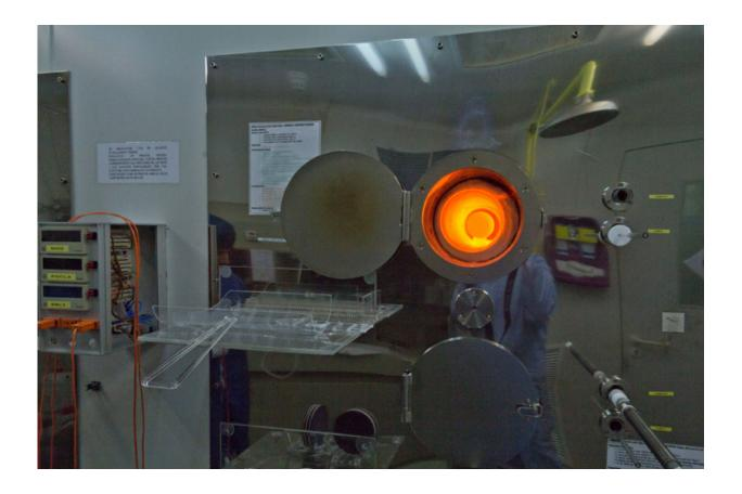
An oxidation oven used in the process of manufacturing black silicon cells
