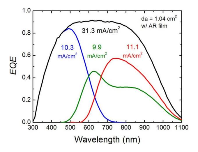
Spectra of the record-breaking triple-junction thin-film silicon solar cell, revealing three different wavelength absorption peaks (or "current densities") that correspond to the three subcells. Credit: Sai, et al. ©2015 AIP Publishing
